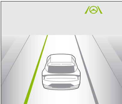
When the front-view camera detects the vehicle moving outside of the lane being traveled in, a yellow marker will illuminate either on the left or right lane (shown in both images above)
