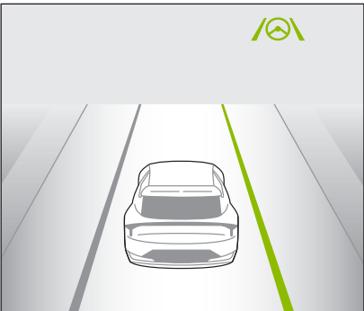
When the front-view camera detects the vehicle moving outside of the lane being traveled in, a yellow marker will illuminate either on the left or right lane (shown in both images above)
