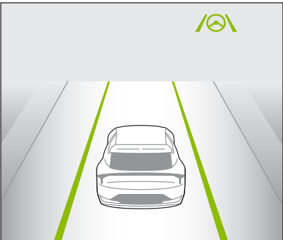
When the front-view camera detects the lane markers, they are displayed white
